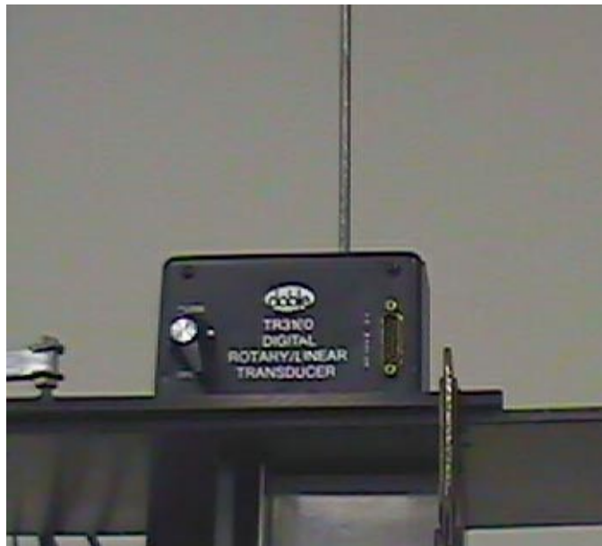
Figure 1.10 Step 3: Linear Motion (Transducer with Rod)
