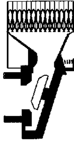
6. Small arcs are attached into loops. This cools the arc and increases resistance to a point where, at an early current zero, the arc is quenched.
